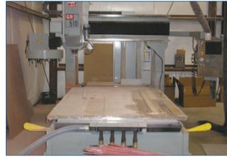
Haas GR510 CNC Router: 3 Routers equipped with custom vacuum tables to aid in quick set-ups.
