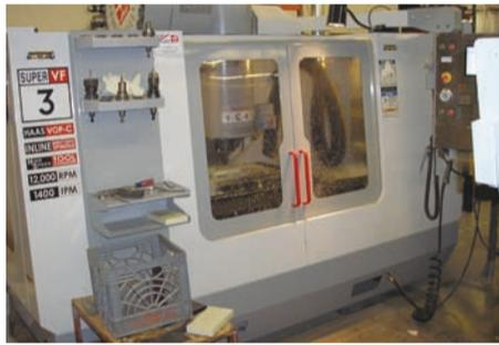
Haas VF3-SS Vertical Milling Machine: 14 Vertical Milling Machines with a maximum working envelope of 40" x 64" x 30."
