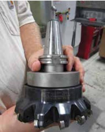
This 6-inch-diameter face mill from Kennametal uses inserts with a titanium diboride ( $TiB_2$ ) coating. Because the coating is thin, it won't dull the insert's sharp cutting edges. However, it still offers the wear resistance needed for glass-filled plastics.
